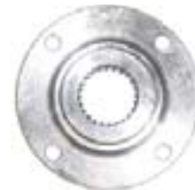
Part# ALT23327 Description (2) Flange coupling 5" 24 spline w/ small seal
