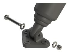
• Unscrew the lower hinge mount of the Lenco actuator from the trim tab by removing the (3) 1/4-20 x 1" long Phillips head screws and nuts using a #3 Phillips head screw driver and a 7/16" wrench.
